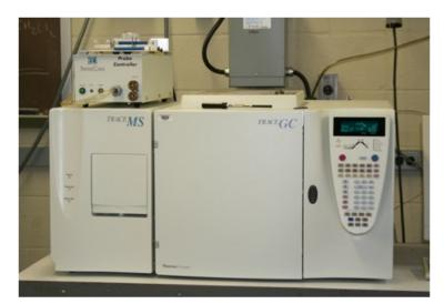
Thermo-Finnigan Trace GC/MS Gas Chromatography Mass Spectroscopy
